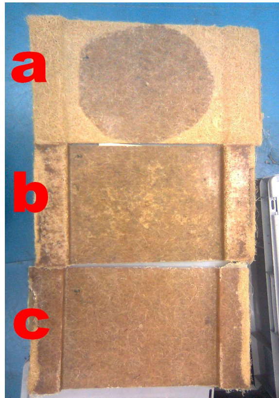
Fig. 2. Results of application of various amounts and types of resin [A) synthetic resin, B) 20% natural resin, C) 10% natural resin]
